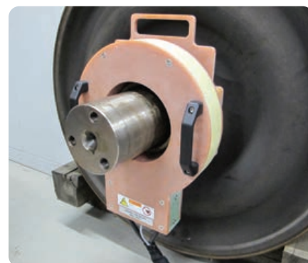
Heating labyrinth rings for dismantling
