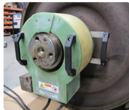
Heating bearing rings for dismantling
