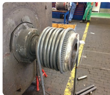
Heating a coupling for dismantling
