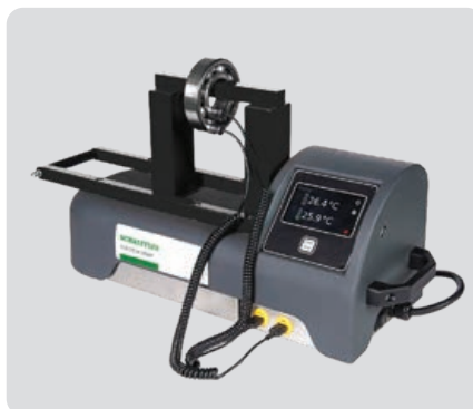
Heating a hanging workpiece, for small bores
